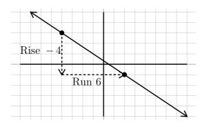
To find the slope of this line we will consider the rise, or verticle change and the run or horizontal change. Drawing these lines in makes a slope triangle that we can use to count from one point to the next the graph goes down 4, right 6. This is rise -4, run 6. As a fraction it would be,  $\frac{-4}{6}$ . Reduce the fraction to get  $-\frac{2}{3}$ .
